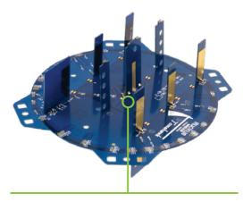
A patented smart antenna array integrates six high-gain vertically-polarized and six horizontally-polarized antenna elements. This enables up to 4096 potential antenna combinations, up to 9 dBi gain and up to 17 dB of interference rejection, thereby delivering unprecedented range extension and signal reliability. The dual polarized smart antenna increases the effectiveness of spatial-multiplexing, resulting in higher data rates.
